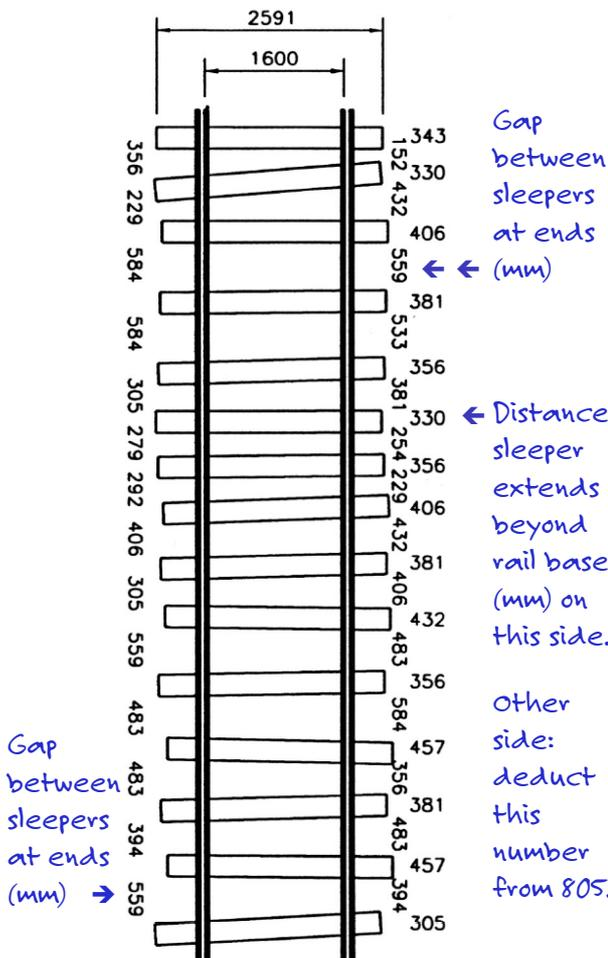
Excluding sleepers adjacent to rail joints: average gap between sleepers 420 mm; average sleeper centre lines 675 mm.
